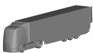
Fig. 2 Aerodynamic truck equipped with air deflectors, side skirts extensions and rear flaps
